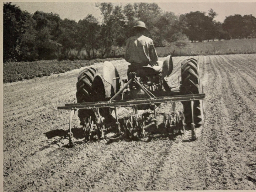
The rotary hoe is very effective for early cultivation. Three 24-inch rows are being cultivated using the rotary hoe attachment and sweep arrangement in the photo above.
