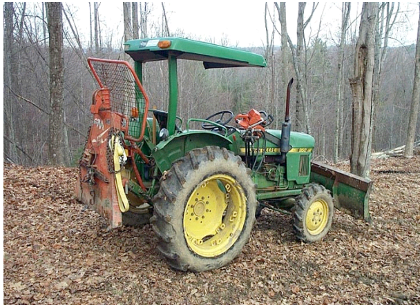
Figure 1. John Deere 950 tractor modified for forestry work
