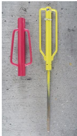
Manual post driver and pilot driver
